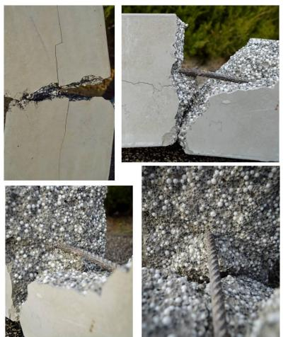
(150\*150\*600) type ICL-K1-PS-LWC with 800 kg CEMII A-S 42.5 N cement and 450 L mixed size expanded PS-beads reinforced with \$\phi 8\$ ribbed reinforcing The steel. "cooperation" between the hardware and the cement frame, typical of lightweight concrete and concrete elements made with ICL admixture in the form of solid granules, is shown in the pictures taken after.
